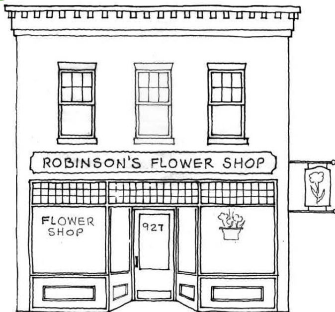
An example of a traditional storefront with transparent storefront and transom windows.
